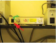
C. Turn on the Multiline argon (457/488/515) laser; 1-turn the power SWITCH on. 2-Then turn the key clockwise to the on position (there is no need to wait for anything here!).
